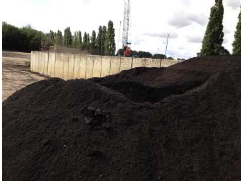
Fig. 15 Stackable final cake with 45% DS after Bucher press dewatering of THP digestion in Chertsey
