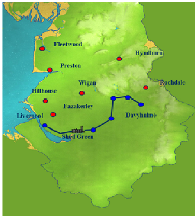
Fig. 7. Layout of 13 WWTPs with Davyhulme digestion and Green Shell Incineration in blue dots and lime stabilization for land use in red dots.
